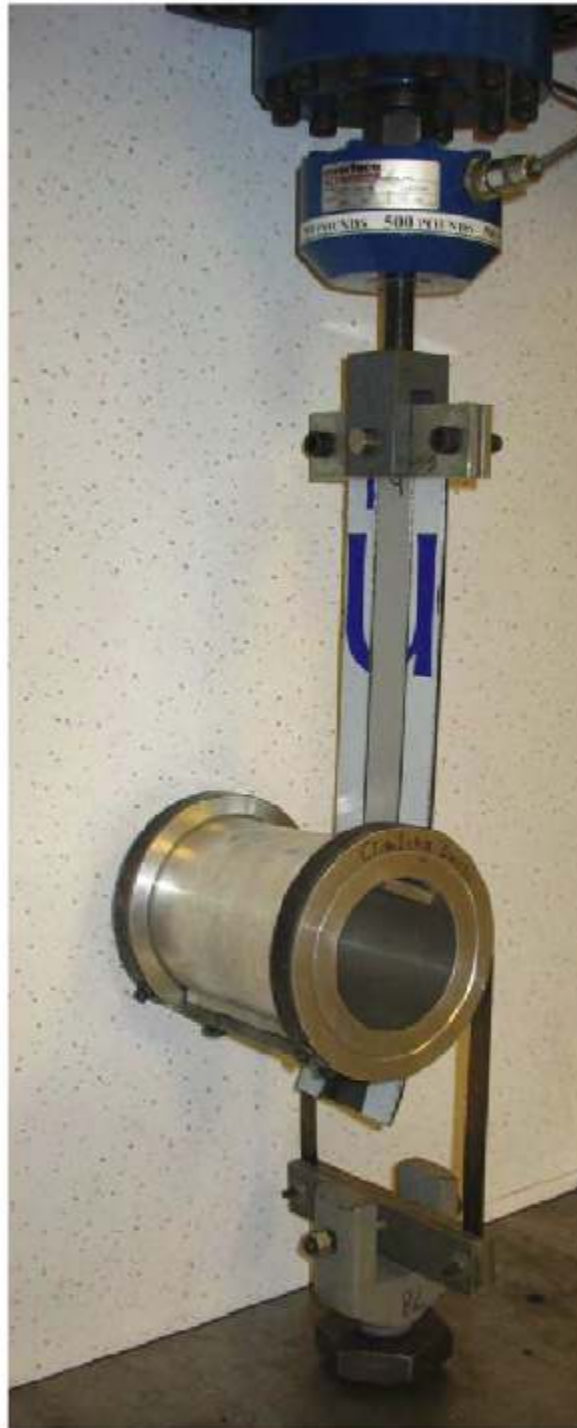
Photo No. 1 Climbing Drum Peel Test - Front View
