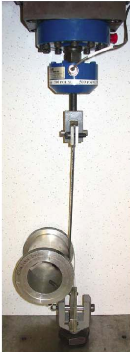
Photo No. 2 Climbing Peel Drum Test - Side View
